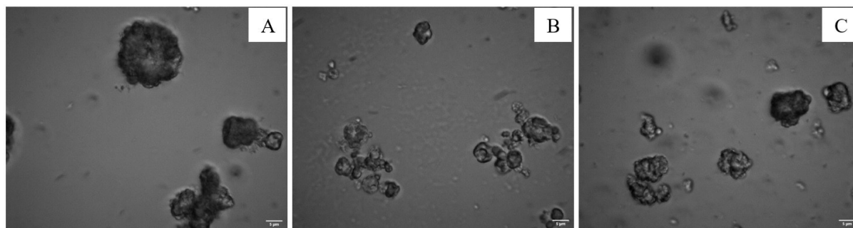
Fig 3: Microphotographs of dry powder of particles encapsulating carvacrol, redispersed in water in following concentrations: (A) 3.35%; (B) 10%; (C) 20%
